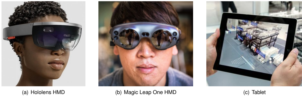
Figure 2.7: Examples of AR HMD's, the bulkier HoloLens (a) and the smaller Magic Leap One (b). Also an AR application running on a tablet (c) ( Images: Tech Stock Insider, Tested, Medium )
