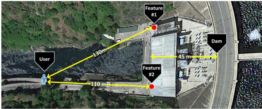
Figure 6.1: Fairly stable tracking is achievable when the user is at about 110 meters from the facade of the power plant (which is situated at around 45 meters from the downstream face of the dam), with a distance between the observer and the tracked Image Target (Feature #1), of approximately 130 meters.
