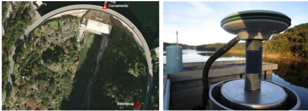
Figure 2.3: Location of the GNSS receivers (left) and detail of the GNSS antenna at the top of the dam (right) [4]
