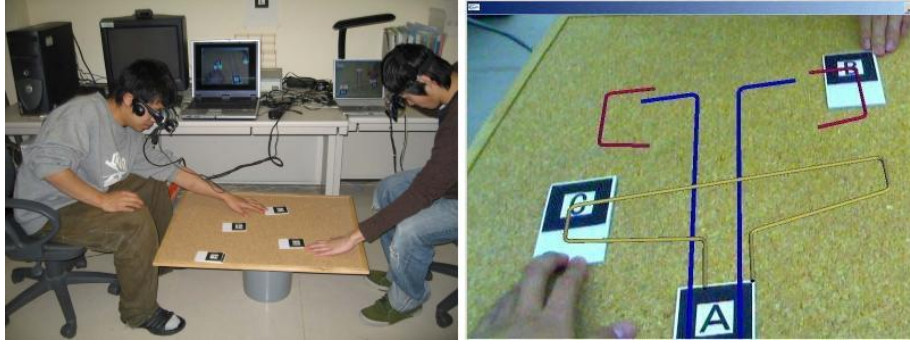
Figure 3.3: Cooperative reinforcing bar arrangement support system using AR technology [29]
