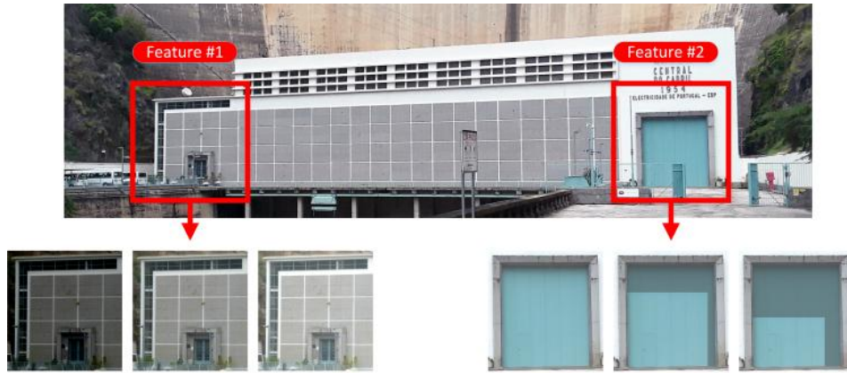
Figure 5.21: The two architectural features chosen and examples of multiple Image Targets with different levels of luminosity and shadow coverage, to improve detection and tracking
