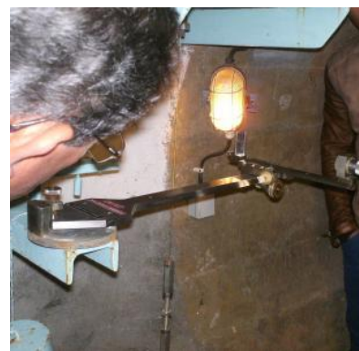
(c) Using an optical coordinometer to read the displacement in a plumbline
