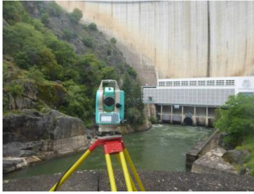
(a) Using a TST to obtain precise space coordinates
