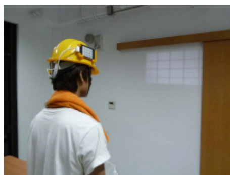
Figure 3.8: BIM data projected directly on building elements [36]
