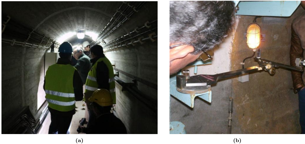
Figure 2.5: Dam safety control experts carrying out an inspection campaign from inside the maintenance galleries of the Cabril Dam in Portugal (a) and using an optical coordinometer to read the displacement in a plumblane (c) ( LNEC ).
