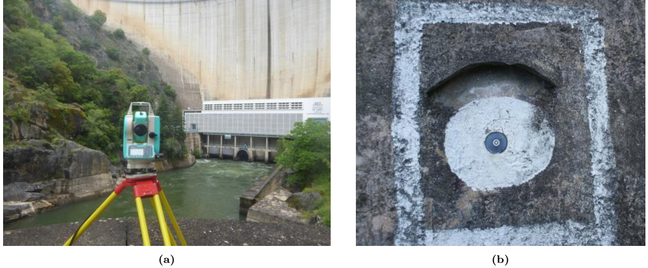
Figure 2.4: Using a total station theodolite (a) to determine the exact position of the fixed geodetic marks (b) installed in the downstream face of the Cabril Dam in Portugal [157].
