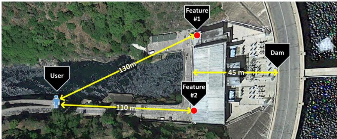
Figure 4.5: During technical visits to the site, a fairly stable operation of the system was achieved at a distance of up to 110-130 meters from the facade of the powerplant (155-175 meters from the dam downstream face) [162], [163].
