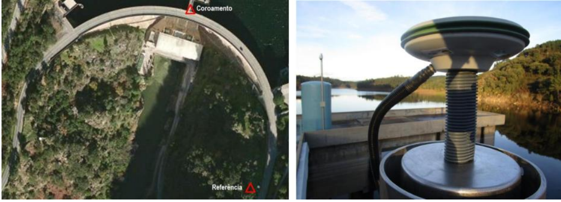
Figure 2.3: Location of the GNSS receivers at the Cabril Dam in Portugal (left) and detail of the GNSS antenna at the top of the dam (right) (LNEC).
