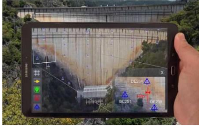
FIGURE 30.7 General view of T1 interface (mockup) shows the menu system on the left and a window panel for zooming in on selected areas of dams on the right.
