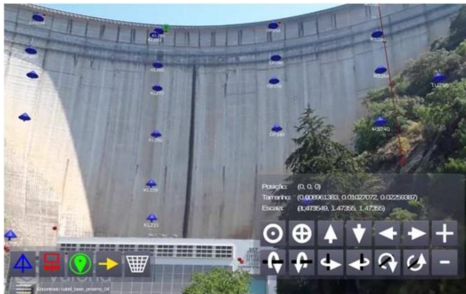
FIGURE 30.8 A screenshot of T1 being used on-site with the sensor network's selected layer (geodetic marks) superimposed on the dam.
